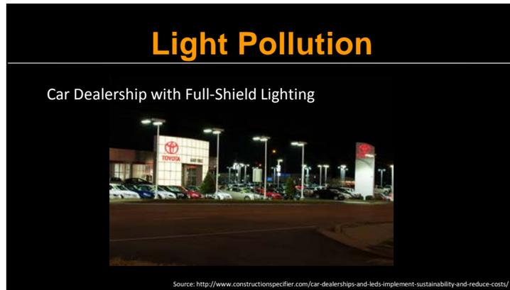
Here is a car dealership that has updated all of its light fixtures to by fully shielding them where all lighting is directed downwards to the ground. Notice that no lighting rises above the top of the lightposts. This result preserves the nighttime sky above the dealership, while keeping the property illuminated.
