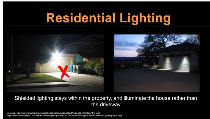
Properly shielded lighting can help lighten up a home, and helps keep it secure. A floodlight above a garage that is pointed towards the driveway and the street creates glare and trespasses outside the property line, and may not always improve security for the house – when the light is projected away, it keeps the house dark. The lights above the garage on the right is cast downward, and illuminates the garage (or wall) of the house, and does not spill over to adjacent property.
