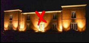
Buildings should be illuminated from the top down, instead of projected upwards. Backlighting and internally illuminated signs are acceptable if set within a certain lumen threshold.
